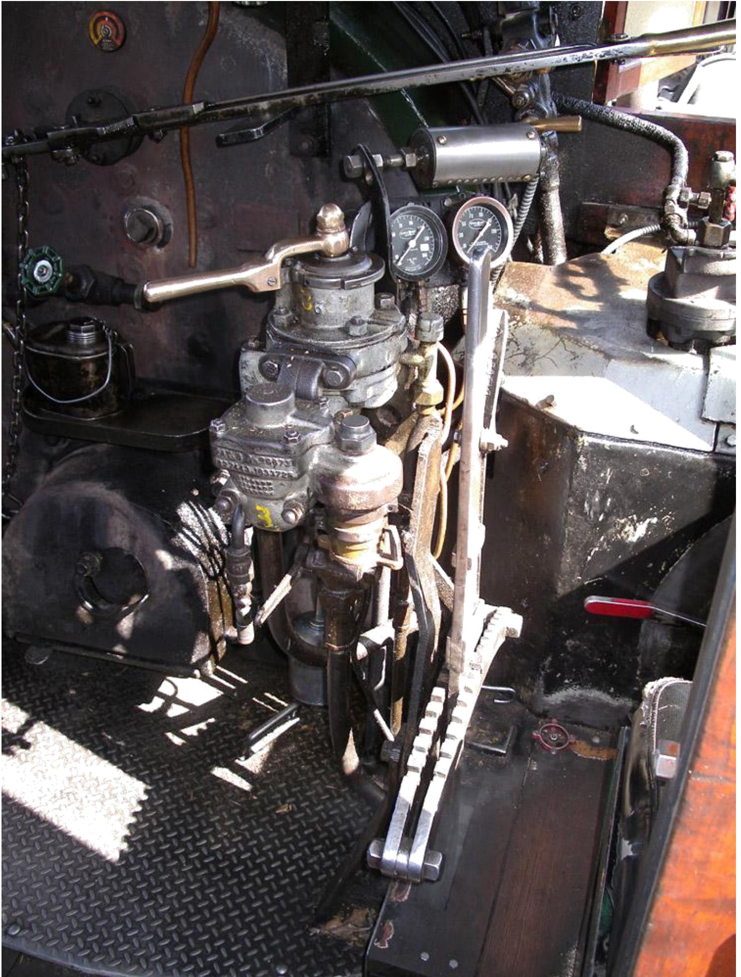
The Johnson bar controls when steam flows into the cylinders
