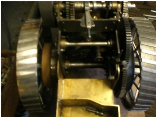
The strakes are simply  $\frac{1}{4} \times \frac{1}{8}$  strips of steel that sit on the outside of the rim at around a  $15^\circ$  angle to the axle as can be seen in the picture looking towards the front of the engine, and their purpose, besides allowing more grip, is to push the wheels towards the centre of the engine as more tractive effort is applied, that way not ripping the wheels away from the axle and the centre of the engine when most power is needed.
