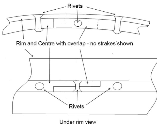
edge, so that with the centre being oversize it will try to push the rim outwards and this means the contact is very close which is something we need to allow the surplus length to be removed.
