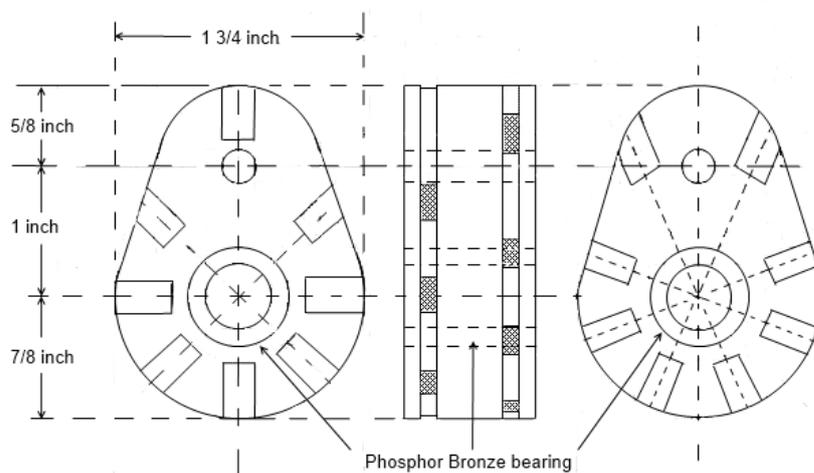
slots are a little offset to each other as can be seen in the drawing, and they are soft soldered together along with the spoke ends once the wheel and hub are built up. It can be silver soldered if you wish, but soft soldering is much easier to accomplish and does the job
