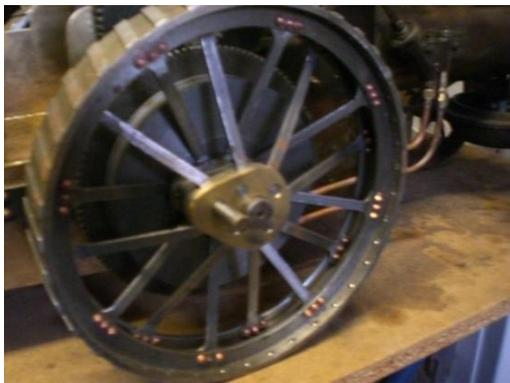
The rim centre is a single piece of steel, unlike this commercially produced rim having two webs along the inside of the rim - but the principal is the same, at  $\frac{3}{8}$  square and a little under 3 feet long (you can use thinner section if you wish providing you are accurate enough with your drilling, as this requires a fair bit of force to bend it to shape, even with heat).
