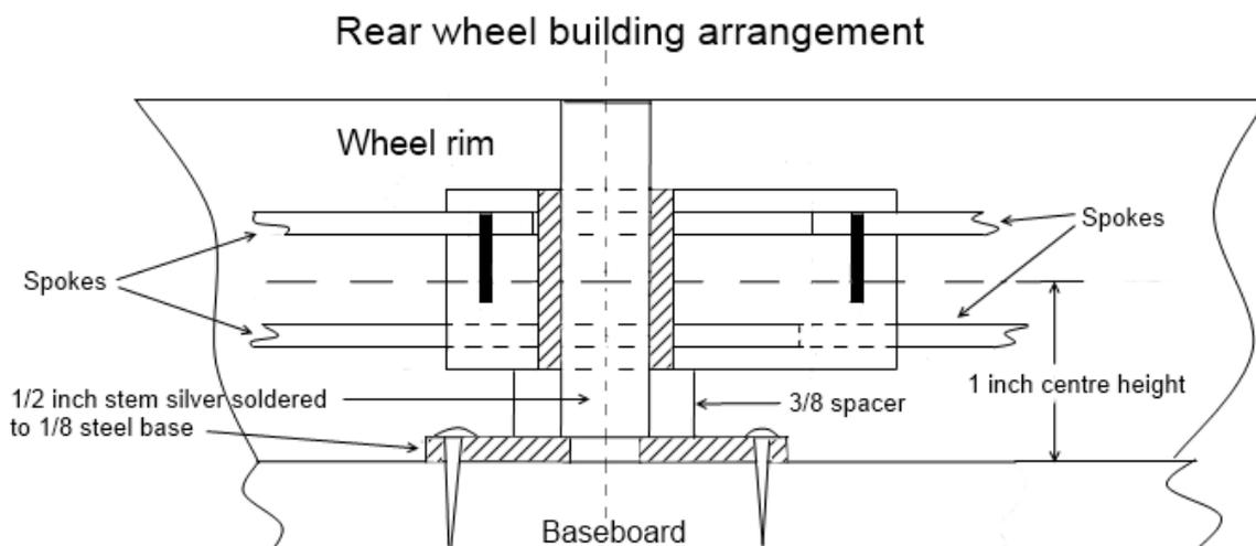
The same  $\frac{1}{2}$  inch diameter pillar is soldered to a  $\frac{1}{8}$  plate as before and this time a  $\frac{3}{8}$  thick packing piece is required to raise the centre of the hub to one inch high from the baseboard surface. You will notice the positions of 2 black  $\frac{1}{16}$  pins showing to secure the upper spokes in place, along with the phosphor bronze bush around the  $\frac{1}{2}$  inch diameter stem.
